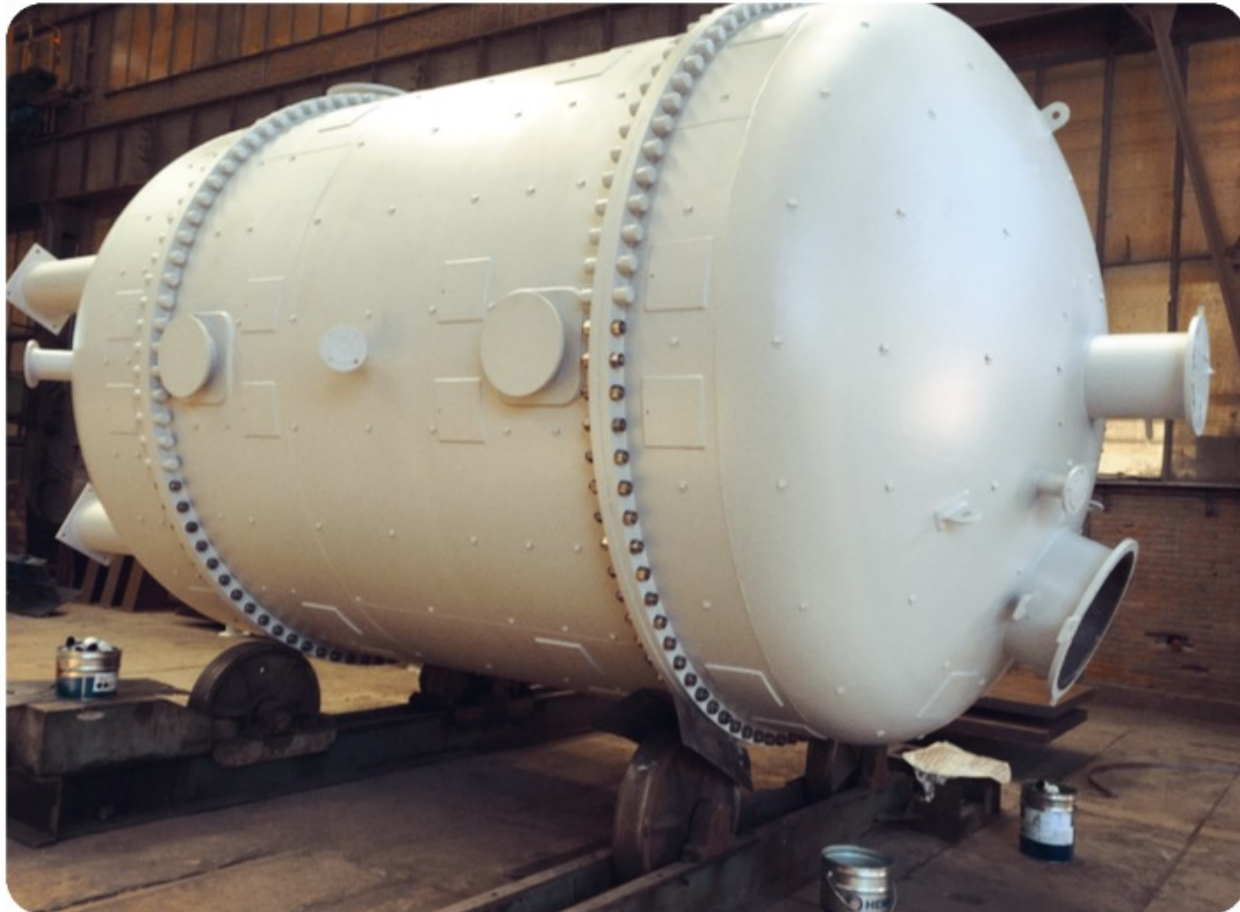
Photo: Industrial installation equipment - Reactor
